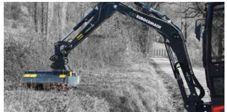
Single/double effect hydraulic system with electrical containment (50 lt/min)
