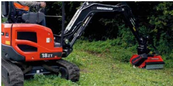
Hydraulic system for chopper with additional pump (19 lt/min)
